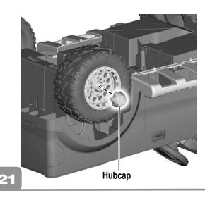
Align the tabs on a hubcap with the slots in a rear wheel. "Snap" a hubcap into the center of the rear wheel.
